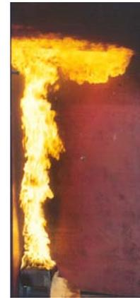
**Figure 4. 300kW Burner for ISO 9705 Test**
