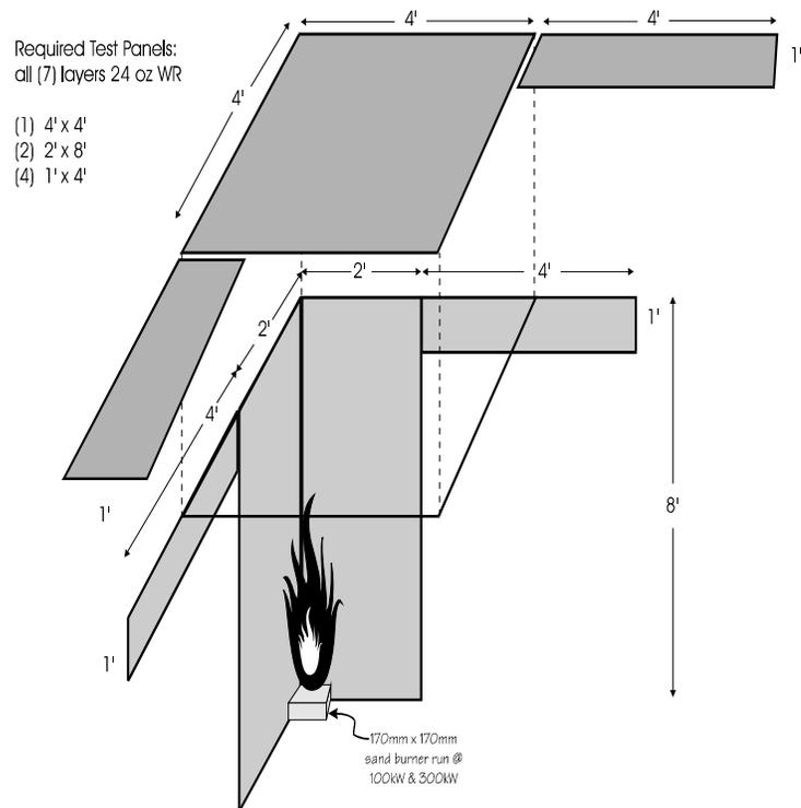
**Figure 5. ISO 9705 Arrangement with Reduced Sample Size using Two 4 x 8 foot Sheets**
