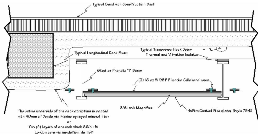
**Figure 8. Typical “A-60” Composite Construction Deck**
