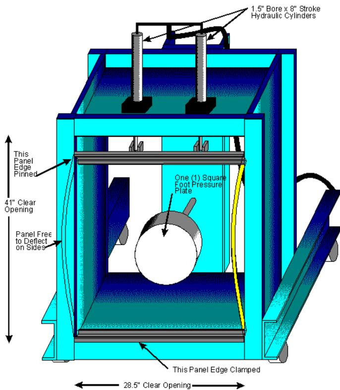
**Figure 6. Multiplane Loading Jig for 3' Samples**
