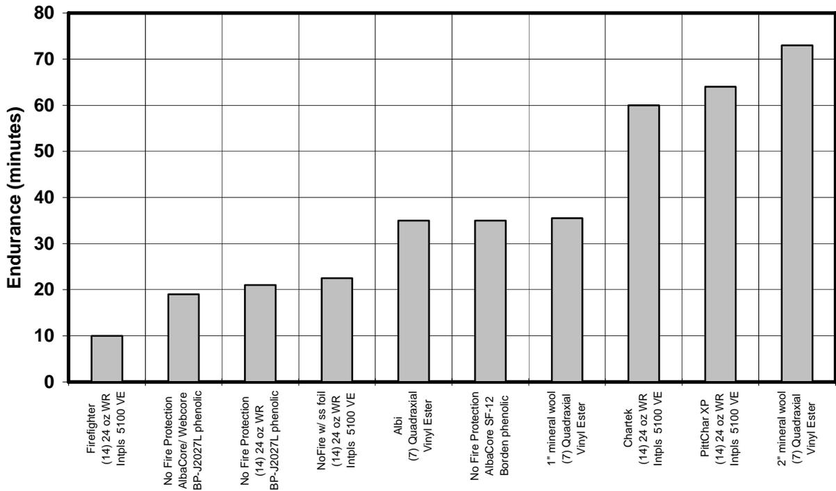
**Figure 7 Burn-Through Resistance of Various Fire Protection Schemes**
