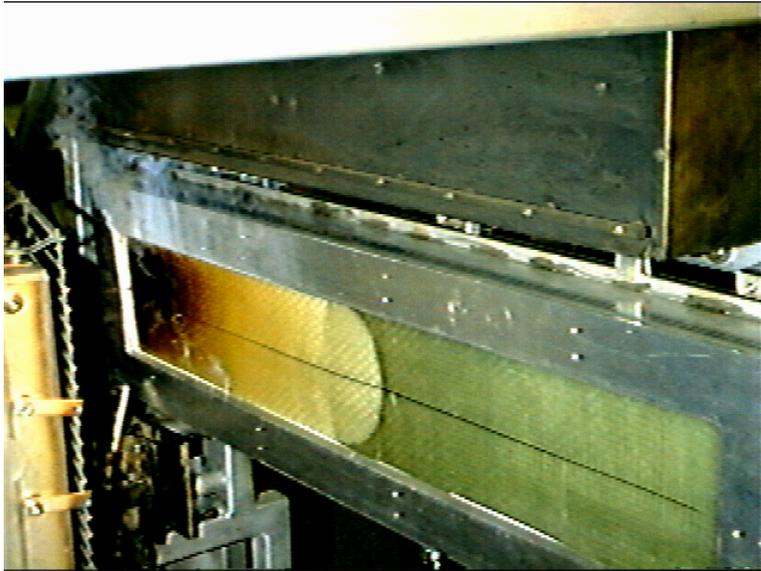
**Figure 3 Flame front Measurement during LIFT Test**
